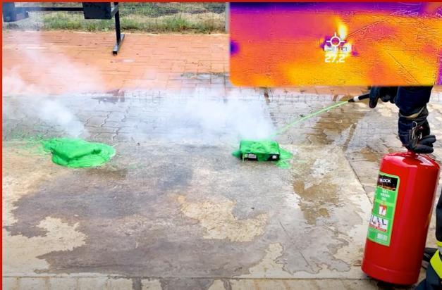
FIREBLOCK LITHIUM comes in the form of fire extinguishers which can be used on small to medium lithium battery fires.
